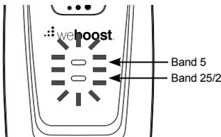
**Green** indicates that the booster is powered and operating at maximum gain.
