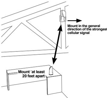
1. Always turn the Outside Antenna so the weBoost logo is toward the strongest cellular signal. The strength of the signal at the Desktop Antenna (and therefore, how far it will transmit a signal) is dependent upon the signal strength at the Outside Antenna. Be sure to maximize the strength at the Outside Antenna.
