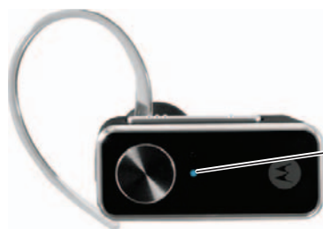
Indicator Light (steadily blue for pairing mode)
