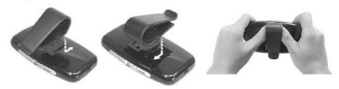
Place the SUPERTOOTH ONE on the sunvisor in such a way that its microphone is directed to the mouth of the user.
