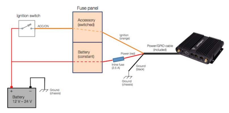
The red power wire requires an inline fuse at 2.0 or 2.5 A. Either use an extra slot in the fuse panel for this fuse, or splice an inline fuse directly into the wiring. Here is an example of how to attach an inline fuse: <u>http://youtu.be/RDOZT-dTITo</u>.
