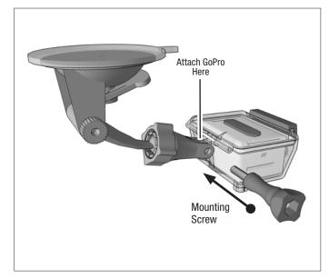
3 Attach mount to windshield and engage suction lock lever. Adjust the mount arm as needed via the adjustment knob.
