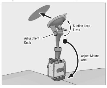
**Optional:** For dashboard mounting, use adhesive dashboard disk. Let dashboard disk adhesive cure for at least 24 hours before use.
