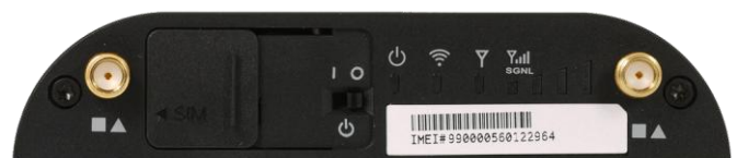
SIM SLOT/ON-OFF / LEDs / SIGNAL STRENGTH COR IBR600
