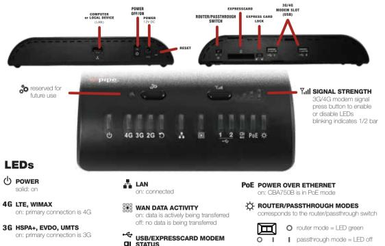
EC green: connected blinking green: connecting amber: not active, may be engaged in failover process blinking amber: connection error blinking red: modem resetting
