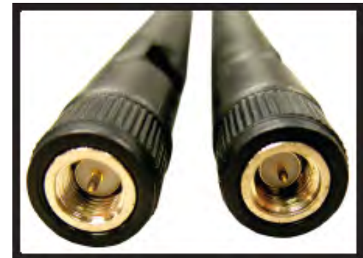
C) Insert antennas (finger tight only).
