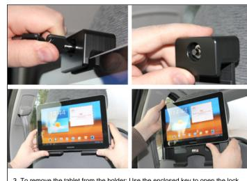
3. To remove the tablet from the holder: Use the enclosed key to open the lock. Remove the lock by sliding it away from the holder. Slide the tablet carefully out of the holder.
