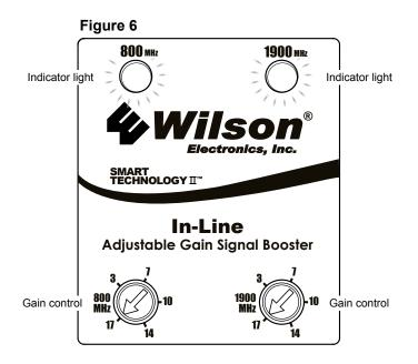
**Note:** If after the initial 15 minutes you are not done with the installation, the In-Line can be reset and enter installation mode again by disconnecting and reconnecting the power supply from the Signal Booster.
