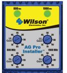
This Signal Booster is supplied with separate uplink and downlink gain controls. Note: All gain controls should be set to maximum. If you have green lights, the installation is complete.
