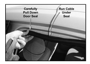
For a more professional-looking installation, the antenna cable may be run under the door seal. Carefully pull down the door seal. Run the cable through the seal and push the seal back into place. This prevents constant wear and tear on the cable as the door opens and closes.
