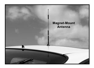
The outside antenna must be installed vertically. Signal performance will be degraded if the antenna is not vertical.
