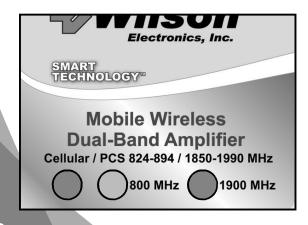
An amber light in either the 800 MHz or 1900 MHz position indicates overload from the cell site. The amplifier has temporarily shut down and will automatically reset.
