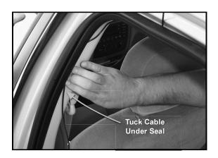
The antenna cable is small enough to easily tuck under the door seal or plastic molding.
