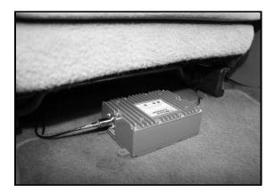
Attach the Cradle Plus cable to the FME-Male connector labeled "inside antenna" on the amplifier.
