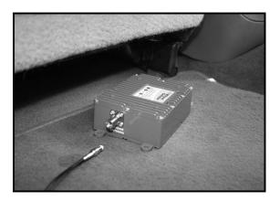
Select a location to install the amplifier that is away from excessive heat, direct sunlight or moisture and that has proper ventilation.
