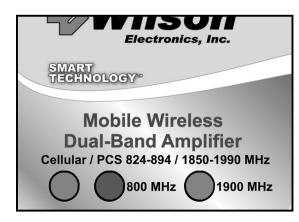
If one or both frequency lights turn red, oscillation is occurring and the amplifier has powered down. The outside antenna needs to be moved farther from the Cradle Plus. Move the outside antenna on the roof of the car to the rear of the car, but at least 8-12 inches from the rear or side windows. Remove power from the amplifier and reinstall power - this resets the amplifier.
