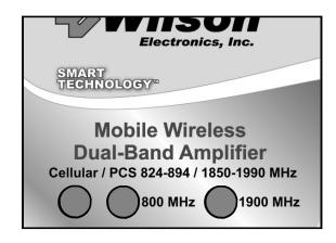
The power light PWR will turn green when the amplifier is successfully powered up. When the 800 MHz or 1900 MHz lights are lit green, the amplifier is amplifying the outside signal.
