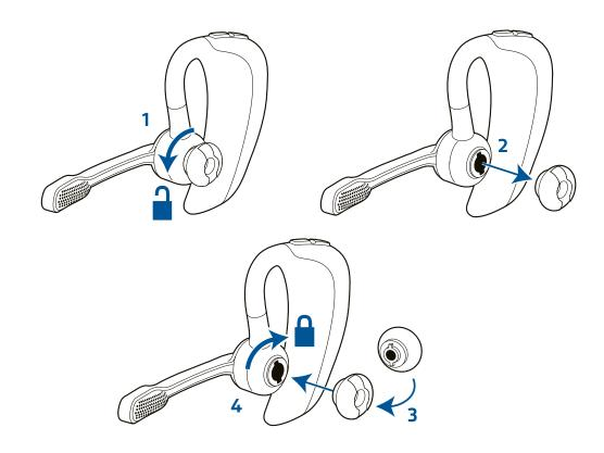
The headset comes with the medium eartip installed, but you can replace it with the optional small or large eartip provided.
