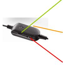
1. To adjust the volume that you hear the other person at, adjust the rolling knob on the side of the pod. Make sure it is on a higher volume setting if you are having trouble hearing the other person.
