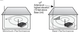
To maximize signal coverage, place the External Antenna where you find the strongest signal (up high or outside) and at least 3 feet above any metal.
