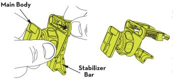
Insert the round end of the spring vent clip into the hole in the middle of the horizontal gap in the Main Body. Slide the Spring Vent Clip to one side and repeat with the other Clip on the other side. Insert the Stabilizer bar into either of the 2 hole sets on the back of the Main Body. (The size of your air vents will determine which set to use.)
