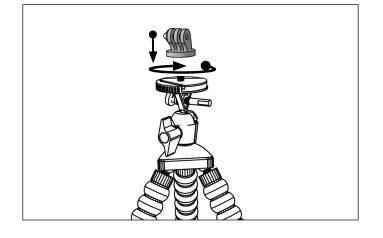
**3** Release the 1/4"-20 mount by unscrewing lateral screw and pressing on release tab.
