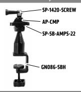
• Attach pedestal clamp by turning the c-clamp knob clockwise; adjust the clamp bracket position if necessary with a Phillips screwdriver. Place ring over ball, attach camera bolt adapter over ball, and tighten to set to position.
