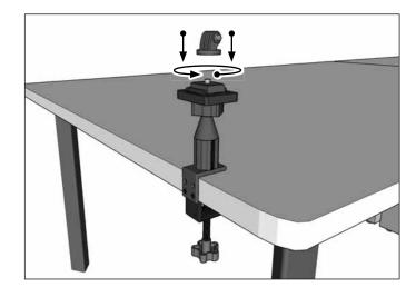
**OPTIONAL:** Release the GoPro mount by pressing on the release tab.
