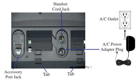
On the right, there is an upper outlet for the Enterprise Telephone handset coil. The lower round outlet accepts the A/C power adapter.
