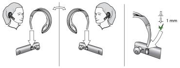
Figure 25: Attaching the ear hook
