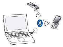
Figure 47: Jabra GO headset paired with both a mobile phone and the Jabra LINK 350 USB Bluetooth Adapter
