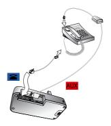
Figure 13.1: Connecting using an electronic-hookswitch adapter (Jabra LINK series)
