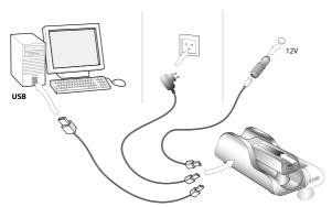
Figure 45: Charging the headset with the Travel Charger
