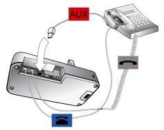
Figure 13: Connecting to a GN1000 Remote Handset Lifter
