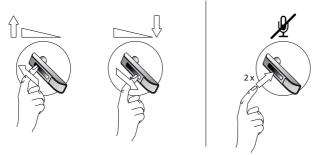
Figure 23: Using the volume strip and mute control
