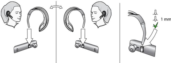
Figure 15: Attaching the ear hook
