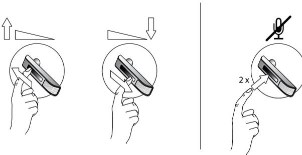
Figure 13: Using the volume strip and mute control
