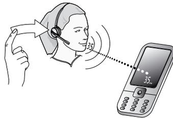
Figure 9: To use voice-activated dialing, tap the multifunction button and speak the appropriate voice tag
