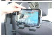
3. To remove the tablet from the holder: Pull firmly on the spring lock so it releases and pull it away from the holder. Slide the tablet carefully out of the holder.
