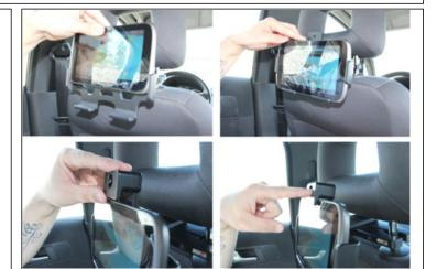
2. To insert the tablet into the holder: Slide the tablet carefully into the holder. Slide the key lock onto the top part of the holder. Press the button in the center of the to lock to secure the tablet in the holder.
