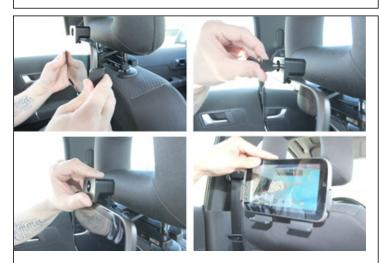
3. To remove the tablet from the holder: Use the enclosed key to open the lock. Remove the lock by sliding it away from the holder. Slide the tablet carefully out of the holder.
