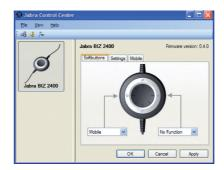
When the headset is connected to your computer, you will see the settings that are relevant for that headset. These settings are divided into three tabs: **Softbuttons, Settings**, and **Mobile** (only when activated). Each of these is described below.
