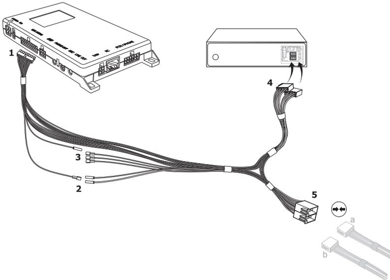
The second red cable coming from the ISO-connectors contains the ignition plus signal (clamp 15). Please connect this with the separate blue cable, whose black Molex connector you subsequently plug into connection 2 on the electronics box. If you are not able to tap the ignition signal via the second red cable, then please check in your vehicle documents and find a different cable which carries this signal.
